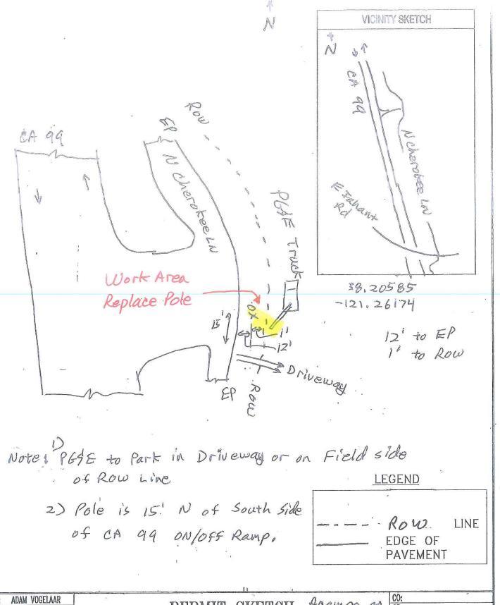
CO: SD: EST: Acampo, CA PERMIT SKETCH Heampe REPLACE DETERIORATED POLE STCO ADE: NOTIF: SUPV: OTHER: REP: E/S N Cherokee Rd 65'5/0 CA 99 Ramp SHT: 1 OF 1 SHEETS PLNR: REV. SCALE: DATF. PACIFIC GAS AND ELECTRIC COMPANY 31193673
